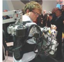
Fig. 2 Multimodal system emerging from an external support which may be a weight compensation system. The final aim of the AIDE project is that such support from the environment disappear when user reaches the assistive structure.
