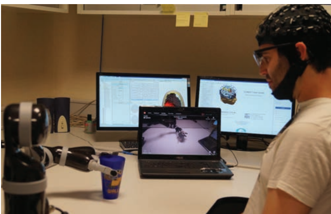
Fig. 1 One of the multiple applications of the AIDE multimodal perception system is a remote control of a robotic device designed for people unable to speak (due to a speech disorder or aphasia) and without functional control of the arm. The multimodal interface will be able to understand the environment and context to automatically recognise the necessary abilities for different activities of daily living. This way, the signals received from the user will be contextualised to interpret the user intentions and execute the desired activity
