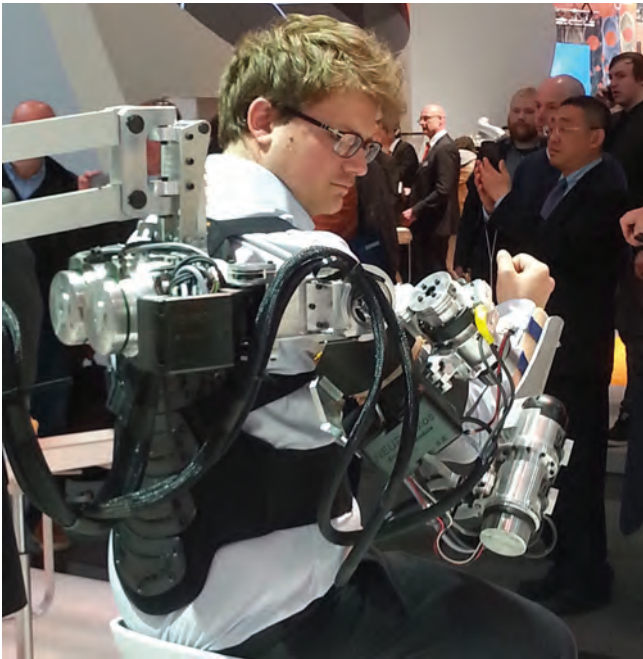
Fig. 2 The AIDE project end product will integrate the NEUROExos system into a support included in a wheelchair structure. Shifting the exoskeleton from an external support with only a weight-compensation system to a portable system will largely improve the applicability of the assistive device and the level of autonomy of the user
